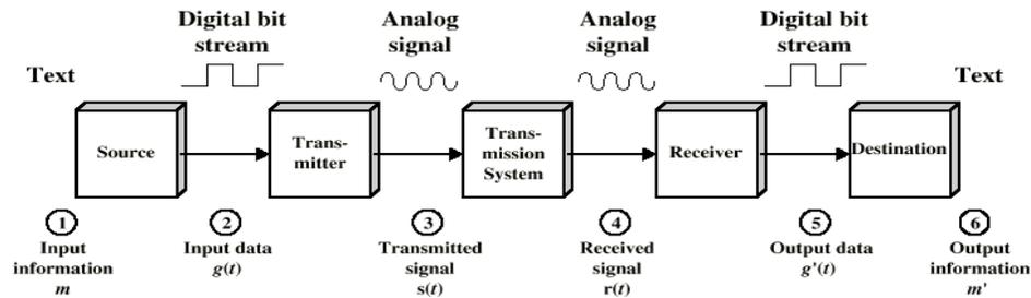
Fig. 1: A simplified data communications model .
